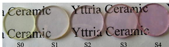
Fig. 1. Photographs of Tm/Er/Yb codoped \text{Y}_2\text{O}_3 transparent ceramic.
